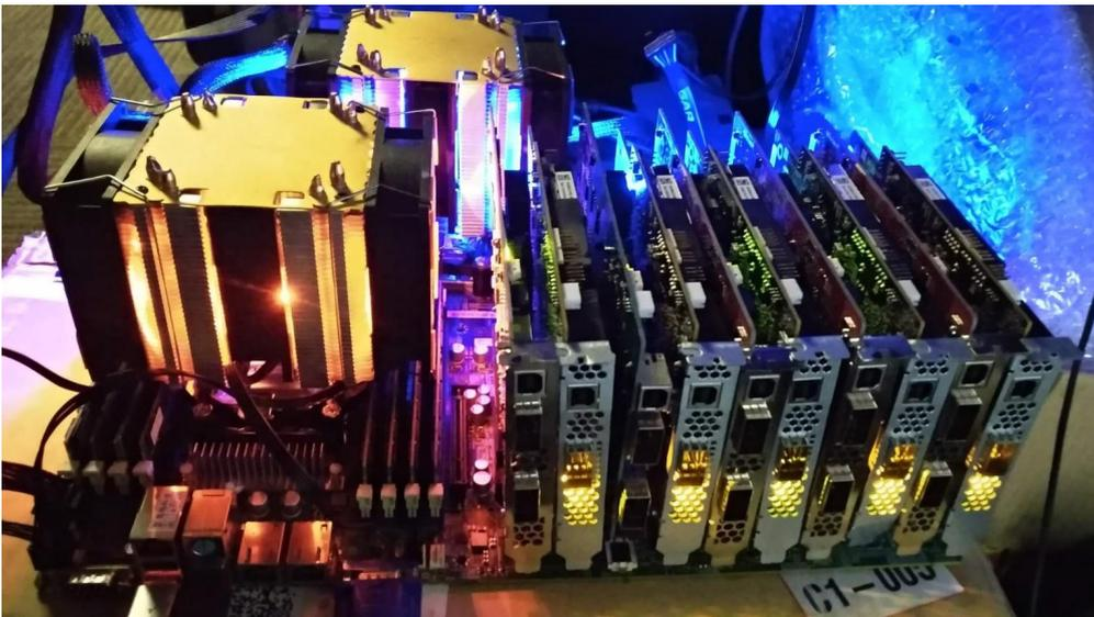
Figure 5.23 10-card KV-Direct system achieving 1.22 billion key-value operations per second at 357 watts power consumption.
